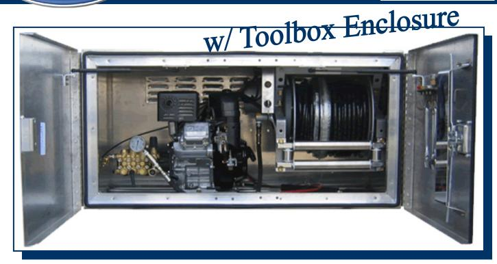
This unit is a very versatile machine and very easy to install. Supplied with a powerful Robins gas engine and a 3000psi rating, the package will do a excellent job with all household lines or grease traps. Grease pumpers find this jetter to be sufficient to provide routine flushing and jetting needs on routine grease trap servicing. The unit only uses 5gpm, allowing its water supply to come from most household faucets.
